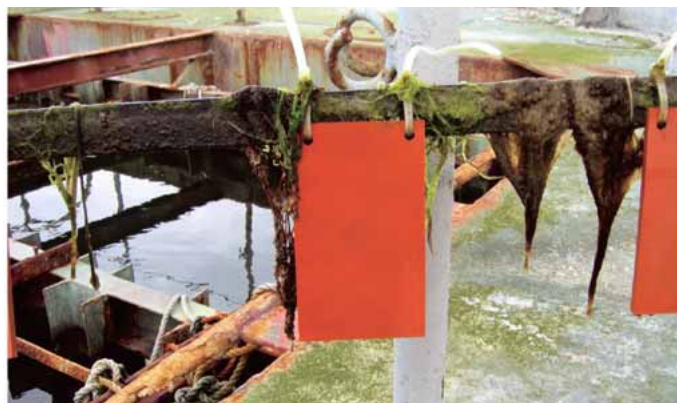
New elastomeric polyurethanes undergoing sea trials off the south coast.
