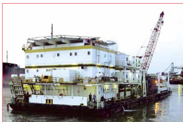
Brazos Horizon, specially designed and built for pipe laying.
