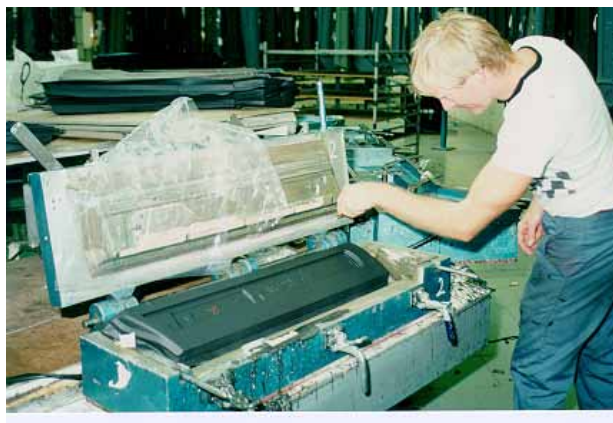
Figure 7 GMFU moulding operation
